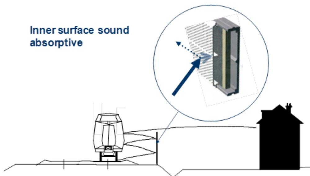
**Graph 6. Illustration of the “canyon”effect and how it can be prevented by an absorptive lining**
